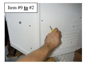
Loosely bolt **Passenger-side Bench/Wall** assembly to 3<sup>rd</sup> **Compartment Bulkhead** using ½" x ¾" Carriage bolts and serrated nuts
